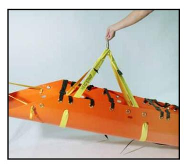
4. EQUALIZE ALL FOUR STRAPS AND SECURE ENDS WITH LARGE STEEL LOCKING CARABINER.
