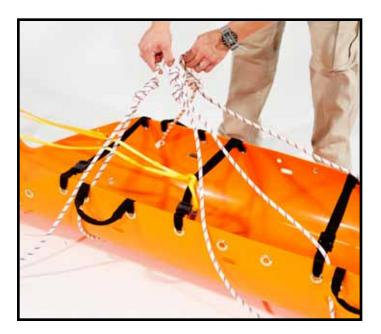
3. TIE FIGURE 8 KNOTS IN BOTH ENDS OF THE ROPE LEAVING ABOUT 2.5 FEET EXTENDING UP FROM THE FOOT END SLOTS AND SHORTER AT THE HEAD END. (SEE PHOTO IN STEP 4)
