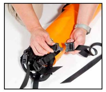
3. WHILE HOLDING YOUR KNEE ON THE ROLLED SKED<sup>®</sup>, FASTEN THE COBRA BUCKLES OF THE FOOT END STRAPS TO HOLD THE SKED<sup>®</sup> IN A TIGHT ROLL.
