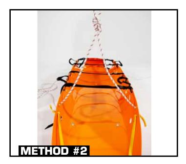
3. FOR EXTREMELY SMALL OPENINGS, LEAVE THE HEAD END EXTENDED. START THREADING THE ROPE THROUGH THE GROMMETS BY THE PATIENT'S SHOULDERS.
